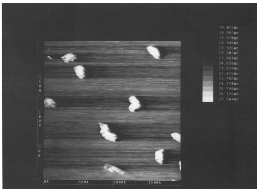
Fig. 6. Round clusters with an average diameter of 200 Å are also observed on the CoMoOx/HOPG sample. These structures are attributed to excess CoOx clusters that did not react with MoOx to form CoMoOx phase.
